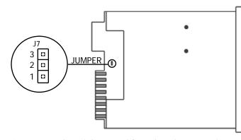
Pin 1 & 2 - For newer style mainframes with anti-arcing protection. Pin 2 & 3 - For older style mainframes without anti-arcing protection.
